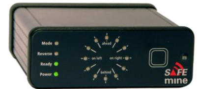
SAFEmine global positioning system technology has been installed in 750 light and heavy pit vehicles.
